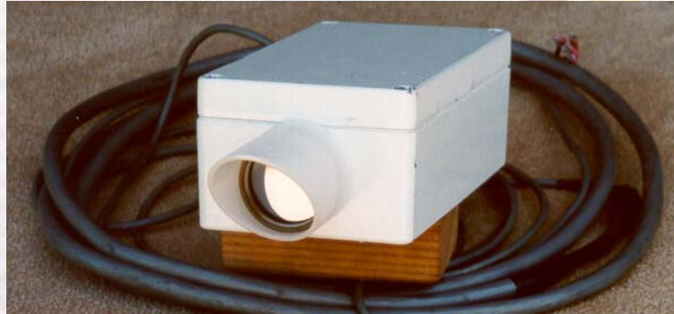
Eltec 842 passive infrared vehicle presence sensor. [ Source: L.A. Klein, Sensor Technologies and Data Requirements for ITS (Norwood, MA: Artech House, 2001) ]
