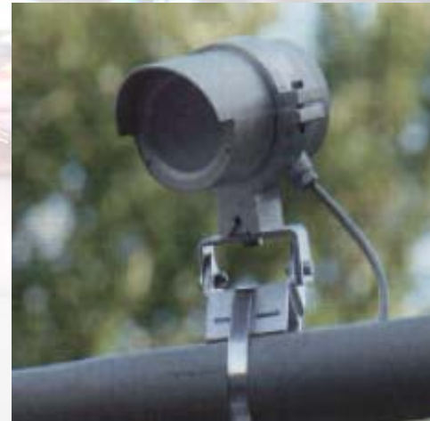
Siemens Eagle PIR-1 sensor. Performs vehicle counting, stop line presence detection, occupancy detection, and queue detection. (Photograph courtesy of Siemens ITS, Austin, TX)
