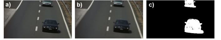
Fig. 3: Original image (a) passed through preprocessing algorithm (b) and after Fg/Bg segmentation (c).
