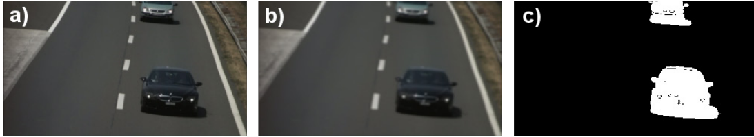
Figure 4: Original image (a) passed through preprocessing algorithm (b) and after Fg/Bg segmentation (c).
