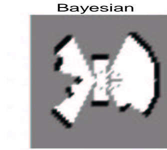
Figure 3: Local occupancy map when robot is in the leftmost position of the corridor given in Figure 4.
