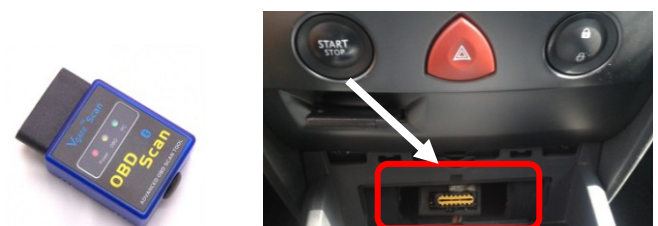
Figure 3. OBD-II Bluetooth external diagnostic device and location of OBD-II port in used vehicle
