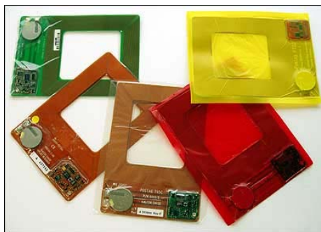
Figure 6. Semi active postal RFID tags
