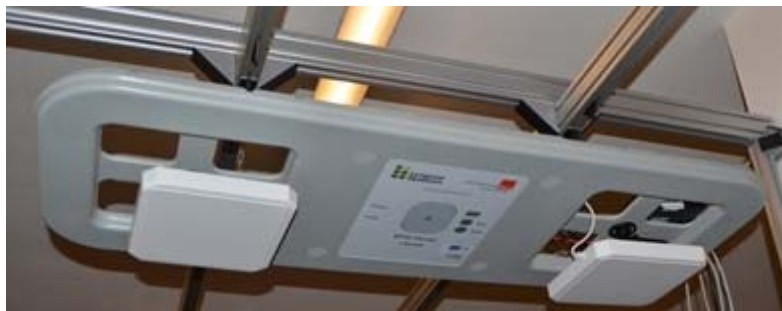
Figure 7. Combine RFID active and passive portal
